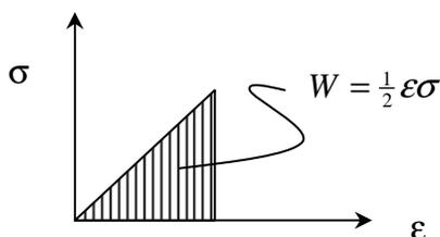
Figure 7.6 : Deformation energy
