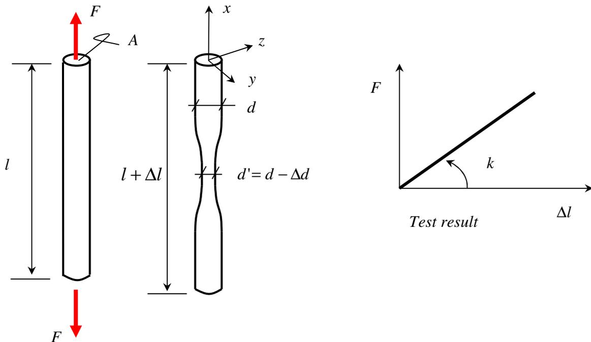
Figure 4.2 : Uniaxial test
