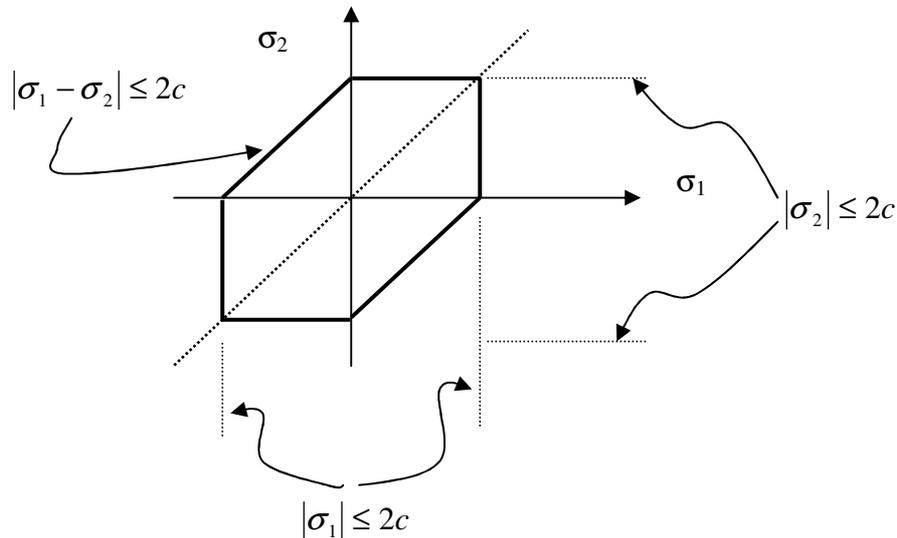
**Figure 6.12 :** Tresca's criterion in the 1-2-principal stress plane
