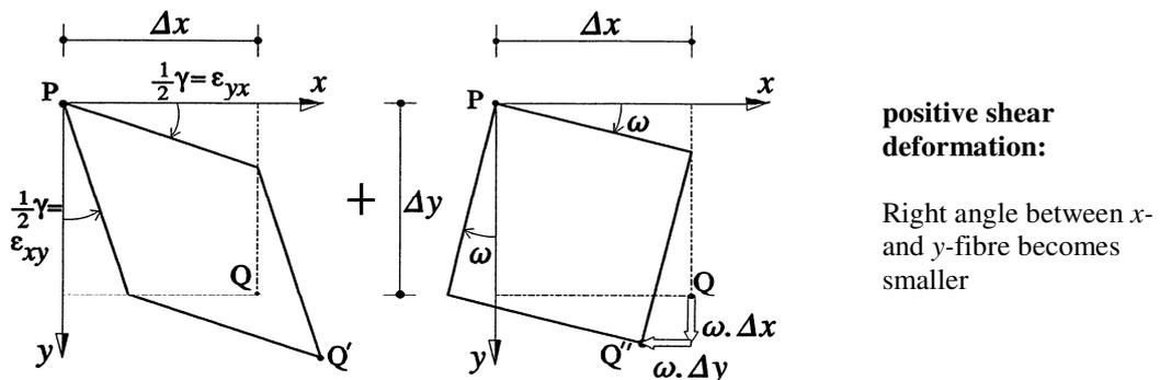
Figure 2.22 : Shear deformation
