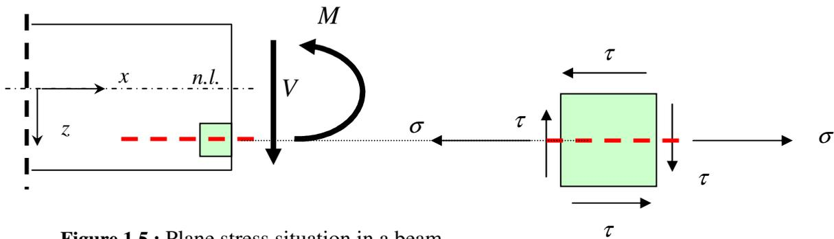
Figure 1.5 : Plane stress situation in a beam
