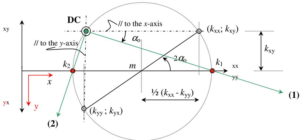
**Figure 2.6** : Mohr's circle, definition of Directional Centre **DC**
