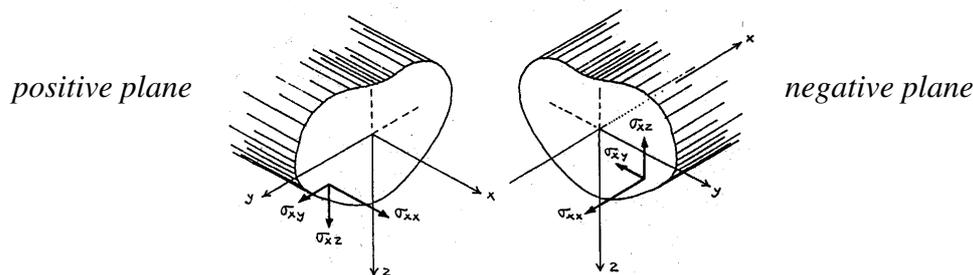
**Figure 1.1** : Normal and shear stresses
