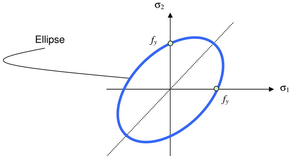
Figure 6.6 : Von Mises criterion in plane stress situation
