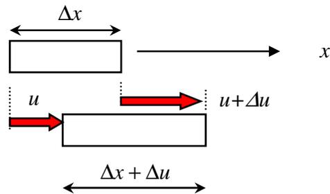
**Figure 1.6** : Strain definition
