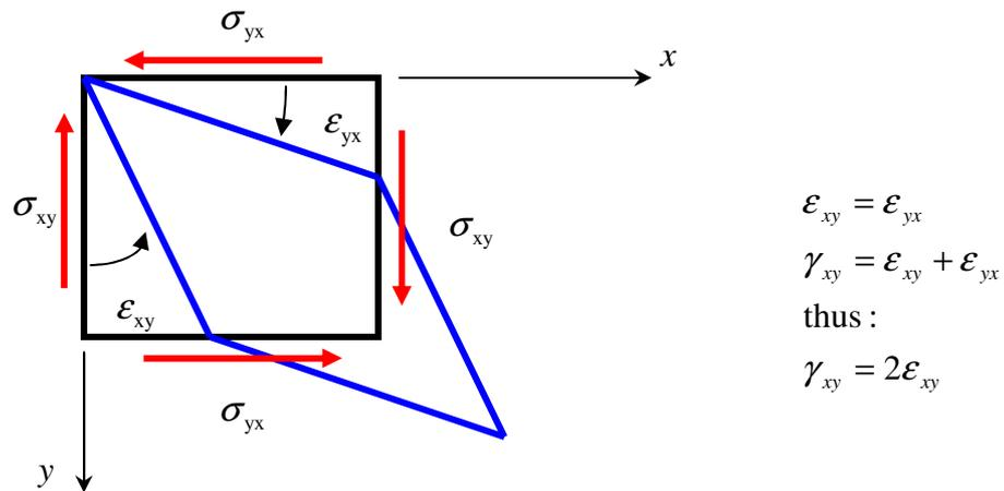
Figure 4.4 : Shear stress and shear deformation in 2D
