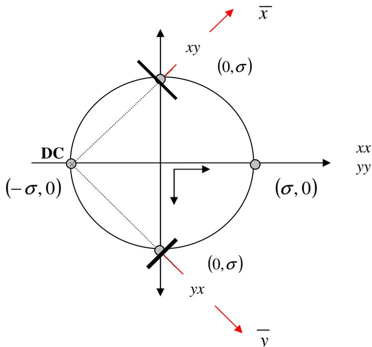
Figure 7.2. : Mohr's circle, pure shear situation
