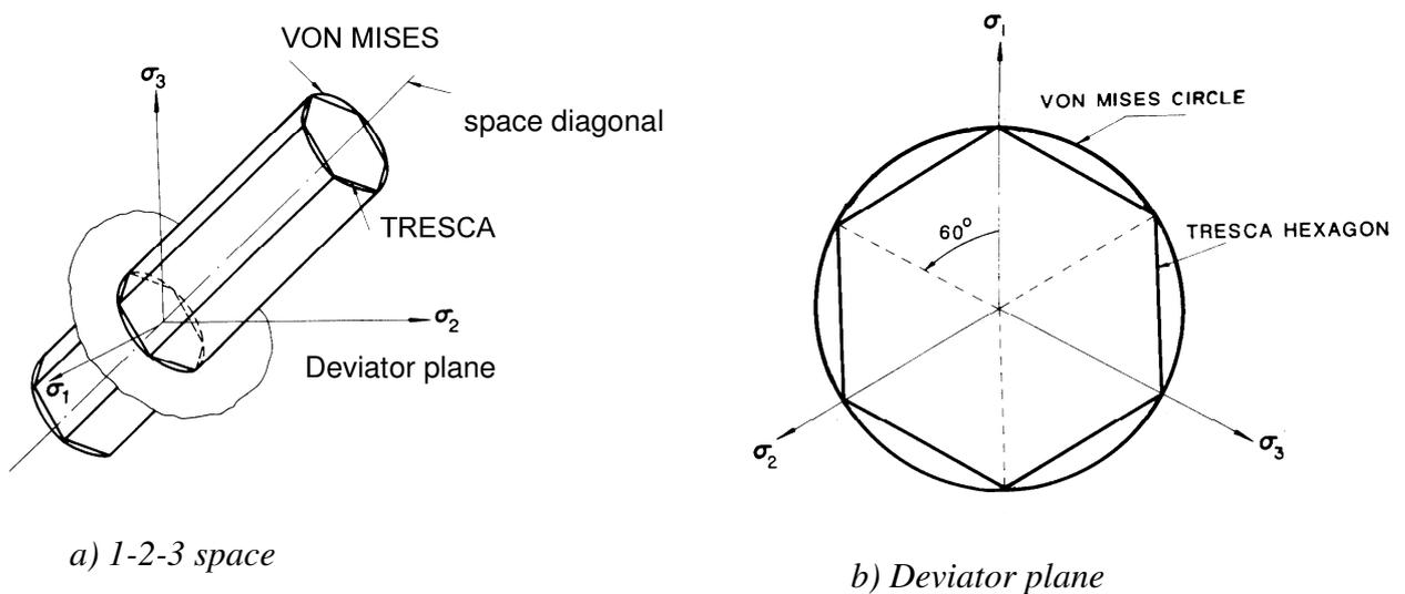
Figure 6.14 : Von Mises versus Tresca
