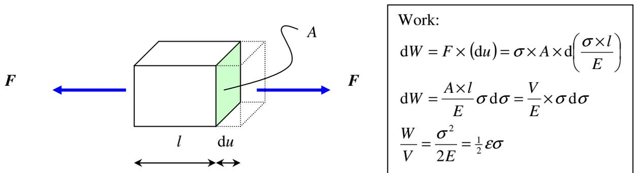
Figure 7.5 : Deformation energy and Work
