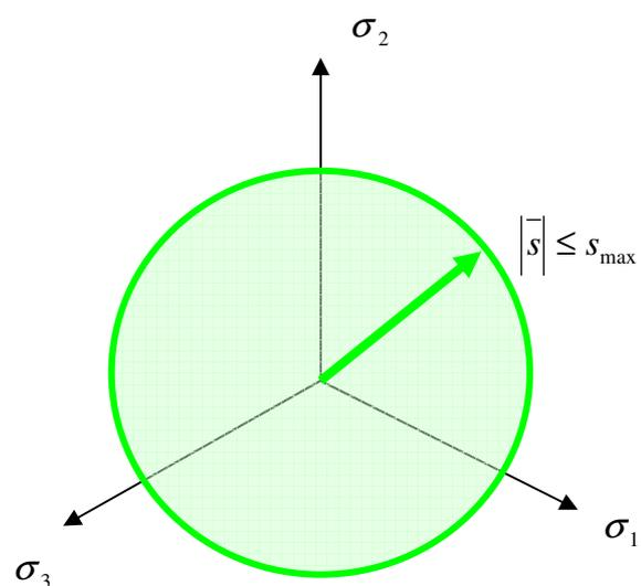
Figure 6.3 : Von Mises criterion
