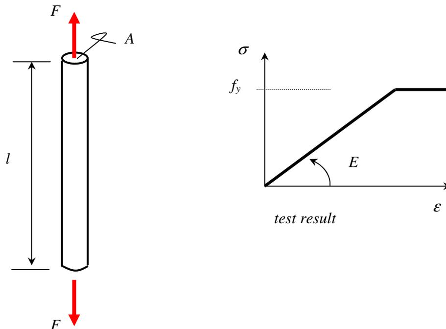
Figure 6.4 : Uniaxial test
