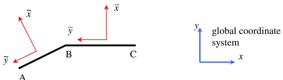
**Figure 2.15 :** Local coordinate system for AB and BC
