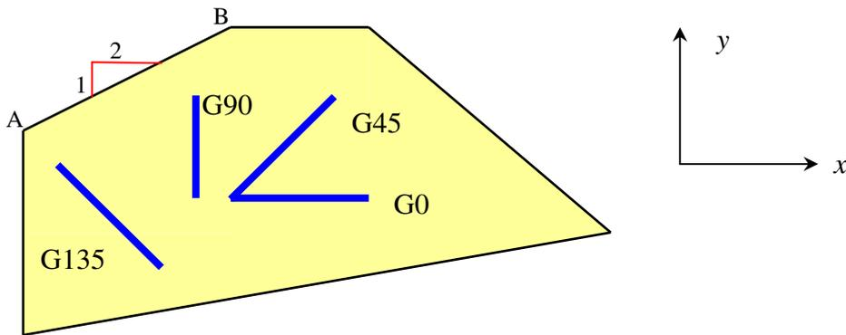
Figure 5.3 : Specimen with mounted strain gauges
