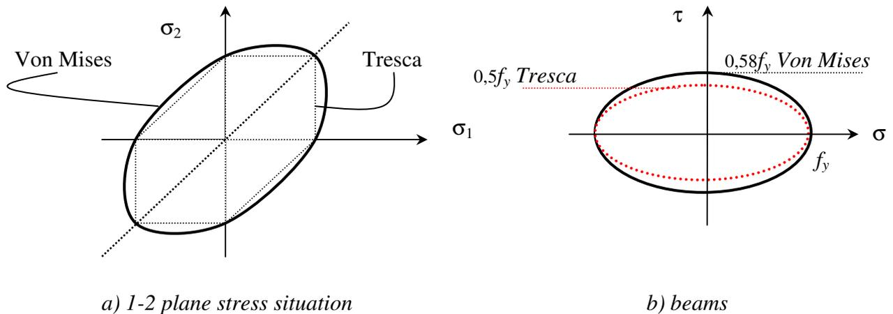
Figure 6.14 : Von Mises versus Tresca (2)
