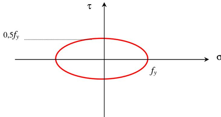
Figure 6.13 : Tresca's criterion for beams in terms of  $\sigma$  and  $\tau$ .
