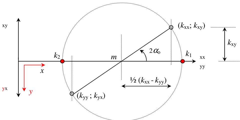
**Figure 2.5 :** Mohr's Circle, definition of coordinate system
