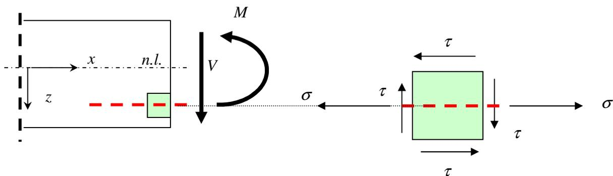
Figure 6.7 : Plane stress situation in beams
