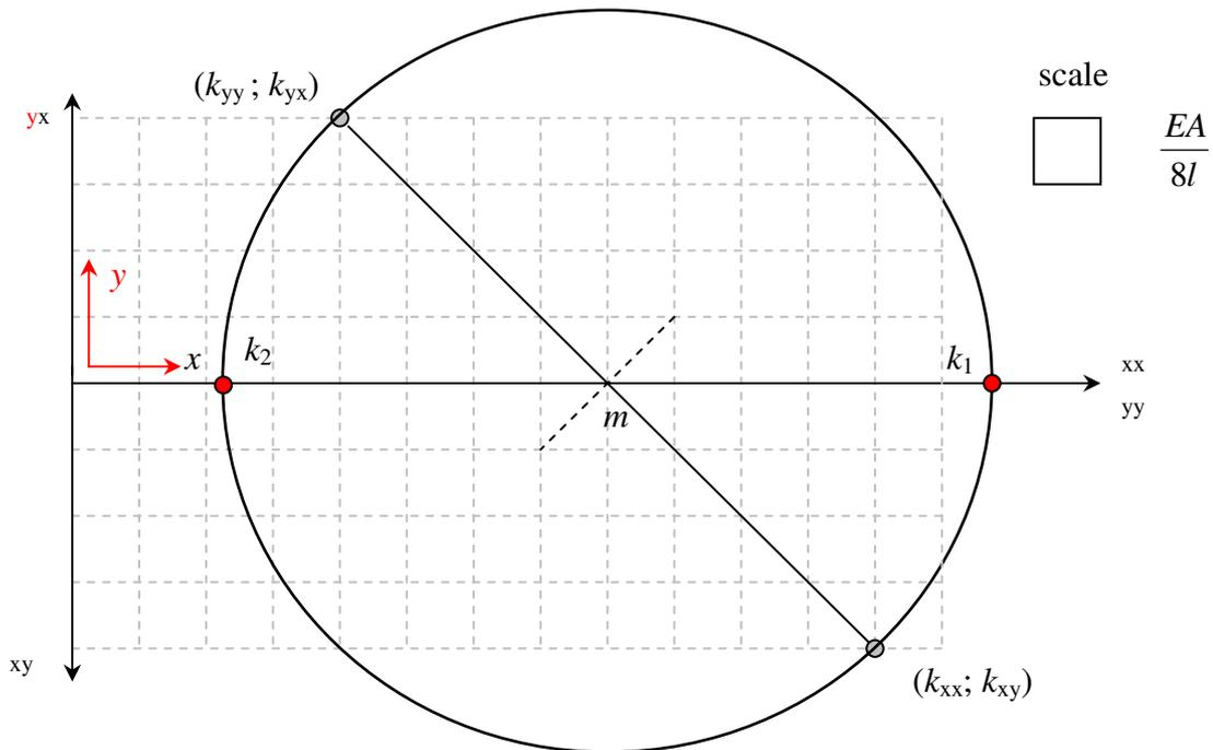
**Figure 2.11** : Mohr's Circle for the stiffness tensor and principal values
