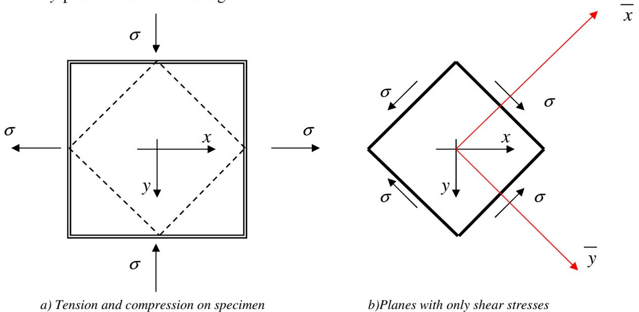
Figure 7.1 : Plane stress with only normal stresses
