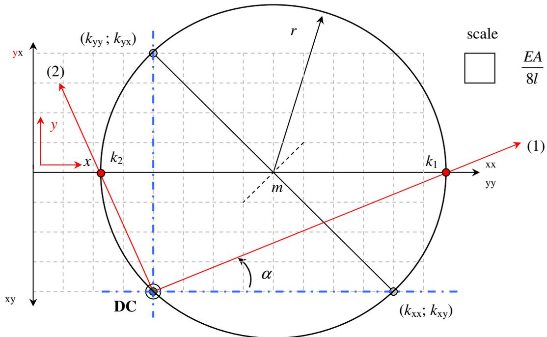
**Figure 2.12** : Directional Centre **DC** and principal directions
