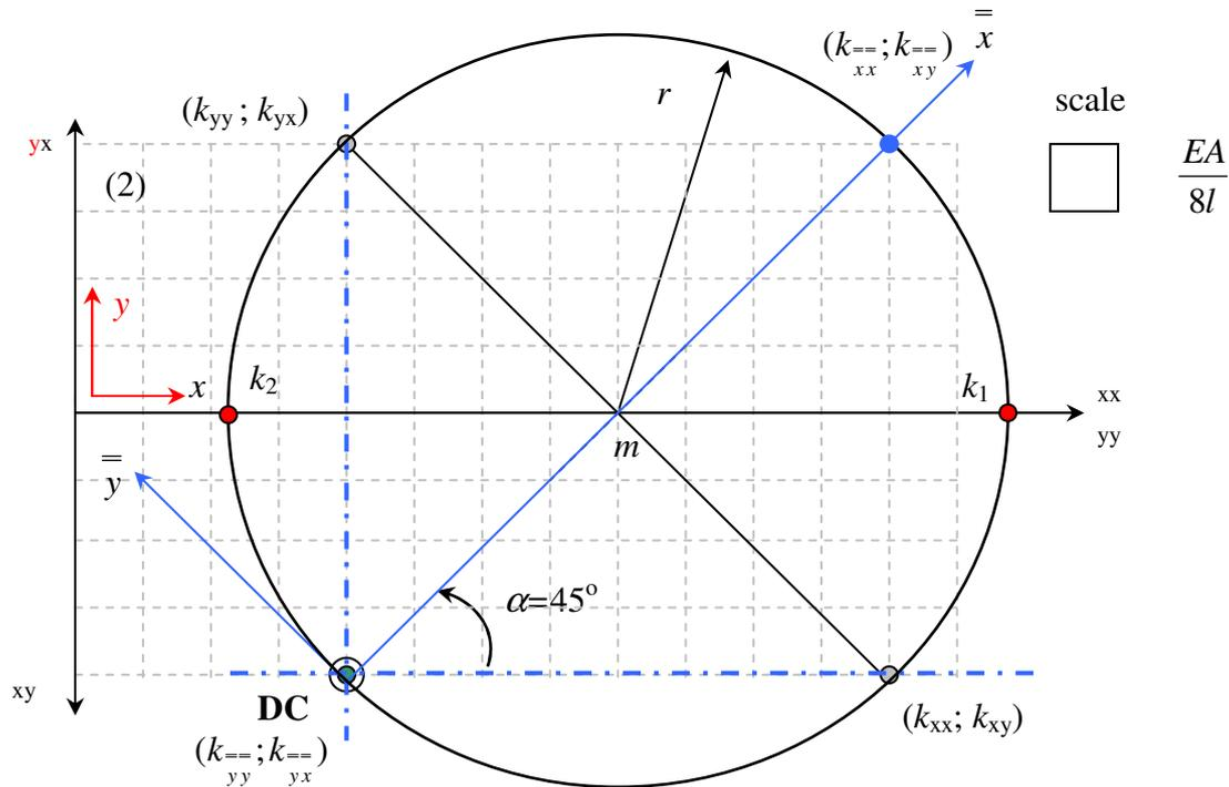
**Figure 2.13 :** Tensor transformation due to rotation of 45 degrees
