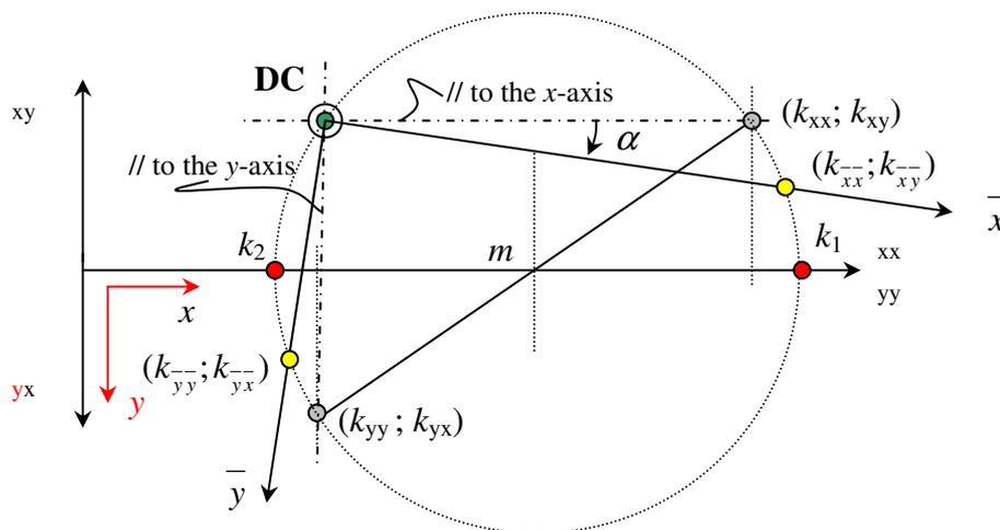
Figure 2.8 : Tensor transformation with Mohr's circle
