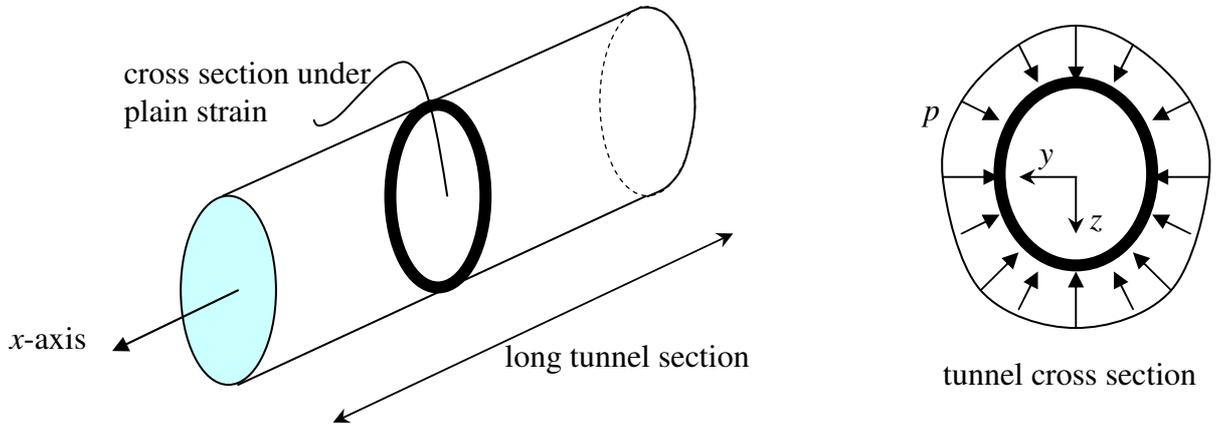
Figure 1.10 : Plane strain situation
