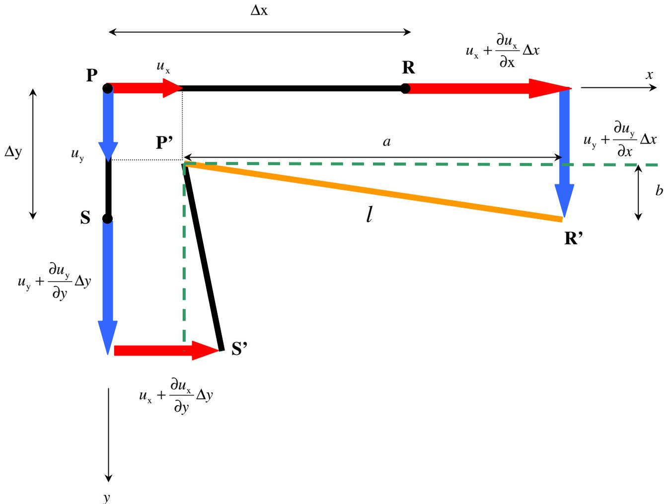
**Figure 1.7 :** Strains in  $x$ - and  $y$ -direction
